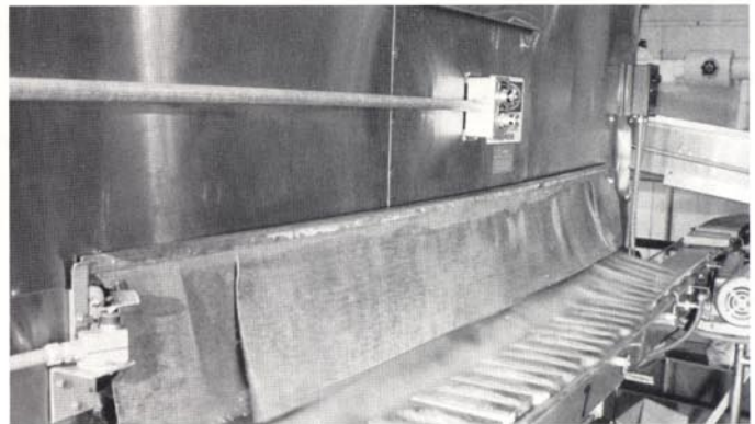
Automatic Discharge Rear of freezer showing frozen product being discharged onto independently driven conveyor assembly.
