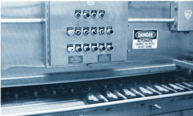
Automatic Infeed Fresh packaged product being conveyed into position just prior to being automatically infeed to the freezer.
