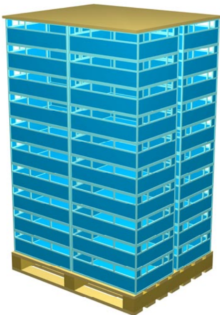
The Pallet - 1200X800 mm Holding Capacity: 40 Trays or 800 kg The trays are self-stacking; a plastic sheet is 'clipped' on top, forming a continuous 'false ceiling' to guide the return air
