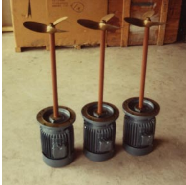
Agitators; with the propellers on extended shafts of flange motors.
