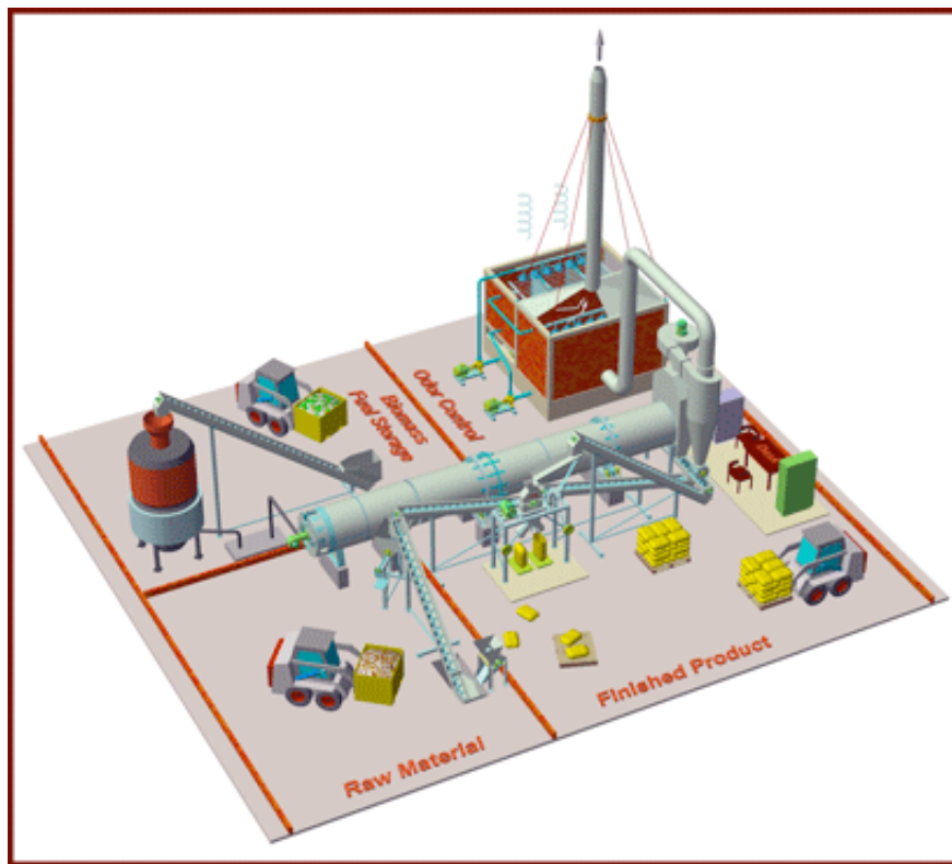
Picture 6 - LeanFish Fish Meal Plant fired with Biomass Gasifier (left behind) (hit the picture for an Acrobat A4 WM (web movie) document - 3,0 MB)
